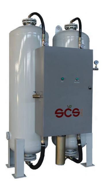
The SCS oxygen system, an on-site PSA oxygen generator, is specifically designed to meet your remote oxygen needs. SCS can supply this series of oxygen systems with capacities up to 2000 SCFH (56Nm3/h), which can be customized with PLC touchscreen or remote cloud operation/data logging.
